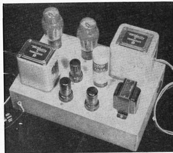
Fig. 45—Appearance of the finished transformer-coupled amplifier.
